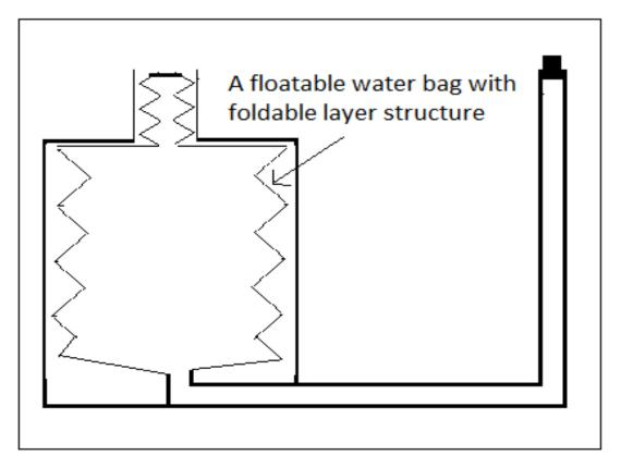
Use a floatable water bag with foldable layer structure as container
