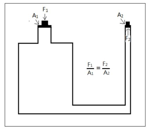
Advantage: Use smaller area to reduce the push-down force needed
