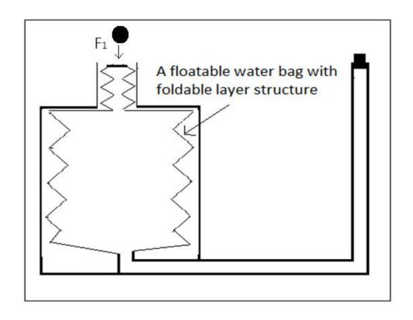
Use a floatable water bag with foldable layer structure as container
